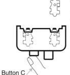
The rectangle and hollow part shall aim at the external part of the door lock, otherwise, the connection pin can't be completely inserted into the hole.
