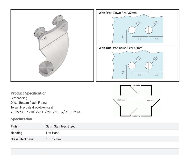
Cut out details for the top & bottom patch fittings are the same, this is not an error top & bottom glass cut outs are the same. The deduction from bottom is to accommodate the H profile drop seal of 21mm is offset exactly by the 21mm height extension.
