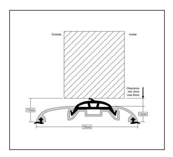
**Product Specification** Suitable for inward and outward opening doors Low profile threshold with concealed fixings Central rubber seal Pre-drilled drainage and concealed fixing holes Ensure door height suitable to meet required 17mm – 19mm
