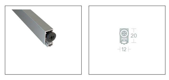
**Product Specification** Application Bottom edge of acoustic timber doorsets Fixing Rebated, held in place with end caps Actuation Single Drop down, maximum 12mm
