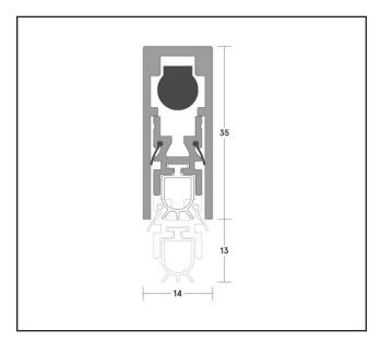
A slimline, face-fixed or semi-mortised automatic drop seal. It features a high efficiency mechanism, which lifts the seal clear of the floor as soon as the door is opened by a few millimetres; resulting in lower door operating forces. Surface mounted application suitable for upgrading existing doors. Requires no power connection. Self-levelling on uneven floors; seal height can be adjusted independently of fixing screws.
