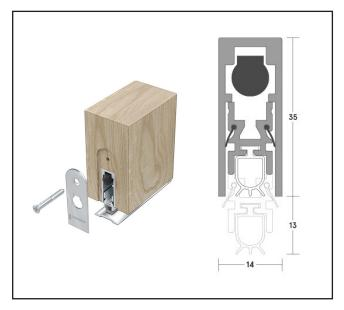
A slimline, mortised automatic drop seal. It features a high efficiency mechanism, which lifts the seal clear of the floor as soon as the door is opened by a few millimetres; resulting in lower door operating forces. Requires no power connection. Self-levelling on uneven floors; seal height can be adjusted independently of fixing screws.
