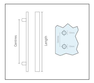
**Product Specification** Includes fixings for glass and timber doors Glass Thickness 10-12mm Timer Door Thickness 44-54mm
