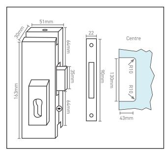
**Product Specification** A centre patch lock for use with frameless glass doors Operated by a euro cylinder (not included) Bolt protrudes 19mm Use our 570.0002.76 glass-to-glass strike for glass side panel applications
