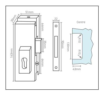
**Product Specification** A centre patch lock for use with frameless glass doors Operated by a euro cylinder (not included) Bolt protrudes 19mm Use our 570.0002.01 glass-to-glass strike for glass side panel applications
