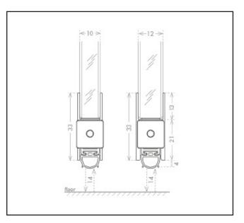
**Product Specification** Can be cut down by a maximum of 150mm Glass Thickness 10/12mm
