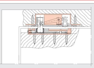
Intumescent gaskets for DORMA double action accessories on **ONE HOUR** timber fire doors.
