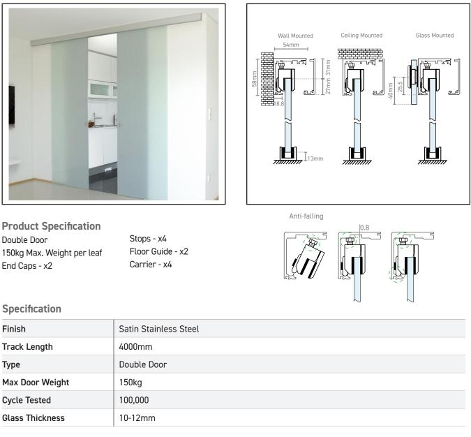
Our new UG sliding glass door system, which covers a wide range of applications and includes options such as soft-close and synchro-opening/closing.
