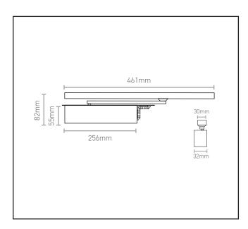
**Product Specification** Fully concealed, adjustable door closer CAM action Meets BS8300 (DDA) requirements Includes Intumescent fire pack FD30/60 Fire tested Includes double action pivot set (FD30/60) which is frame mounted
