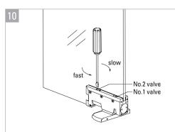
Door closing speed adjustment from  $90^{\circ}$  -  $30^{\circ}$ , loosen No.1 valve counter-clockwise to speed up, tighten No.1 valve clockwise to slow down. 1 mm higher than the hole is prohibited while adjusting No.1 valve.
