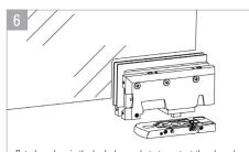
Put glass door in the body, lay gaskets to protect the glass door on both sides, use Allen key to tighten the 4 hexagon socket countersunk head screws on spring body to fix the glass door.
