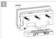
Mount the body on the base, choose suitable gaskets per glass door thickness, loosen the 4 hexagon socket countersunk head screws on body to install the glass door.
