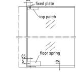
When used with top patch or top pivot, pivot center must be aligned with floor spring pivot center. Determine the top & bottom shaft center and the installation position for base, keep suitable gap on the side as picture shows.
