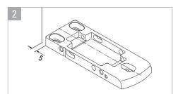
To determine the base installation position, keep a 5 mm gap from the side and draw lines to mark the 3 mounting positions.
