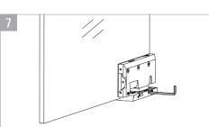
Use Allen keys to tighten the set screws on both sides of the base.
