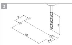
Drill 3 holes with diameter 10 mm, depth 68 mm at the marked mounting positions.
