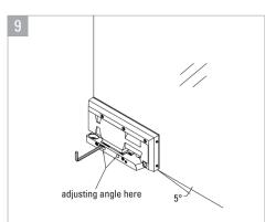
To adjust the glass door angle finely by adjusting the set screws on the movable block sides as picture shows per actual needs.
