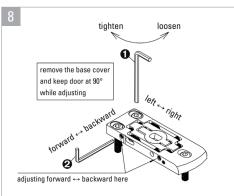
As picture shows  $\odot$  to adjust the base left and right by loosen 3 hexagon socket head cap screws  $\odot$  to adjust the glass door backward and forward by adjusting the set screws on base sides.
