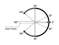
Door closing speed adjustment from 30° - 0°, loosen No.2 valve counter-clockwise to speed up, tighten No.2 valve clockwise to slow down. 1 mm higher than the hole is prohibited while adjusting No.2 valve.
