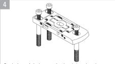
Put the inner pin in the expansion dowel, then place the expansion dowel in the mounting hole.
