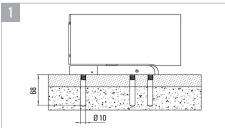
Use hexagon socket head cap screws and threaded expansion tube for brick and cement floor, use self tapping screws for wooden floor.
